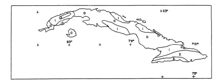
Figure 1: Seismic zones for seismic building code NC-53-114. O-I < VI, 1 - I = VI, 2- I = VII, 3 - I = VIII.
